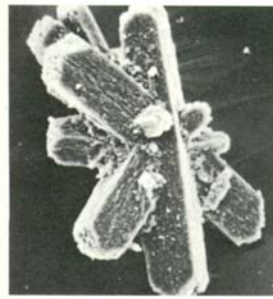
Figure 5.6 Electron micrograph of a cluster of phillipsite crystals recovered from Pacific deep-sea sediments. Scale bar 25µm. The formula of phillipsite is (K,Na,Ca)_3(Al_3Si_6O_{18}) \cdot 6H_2O .
