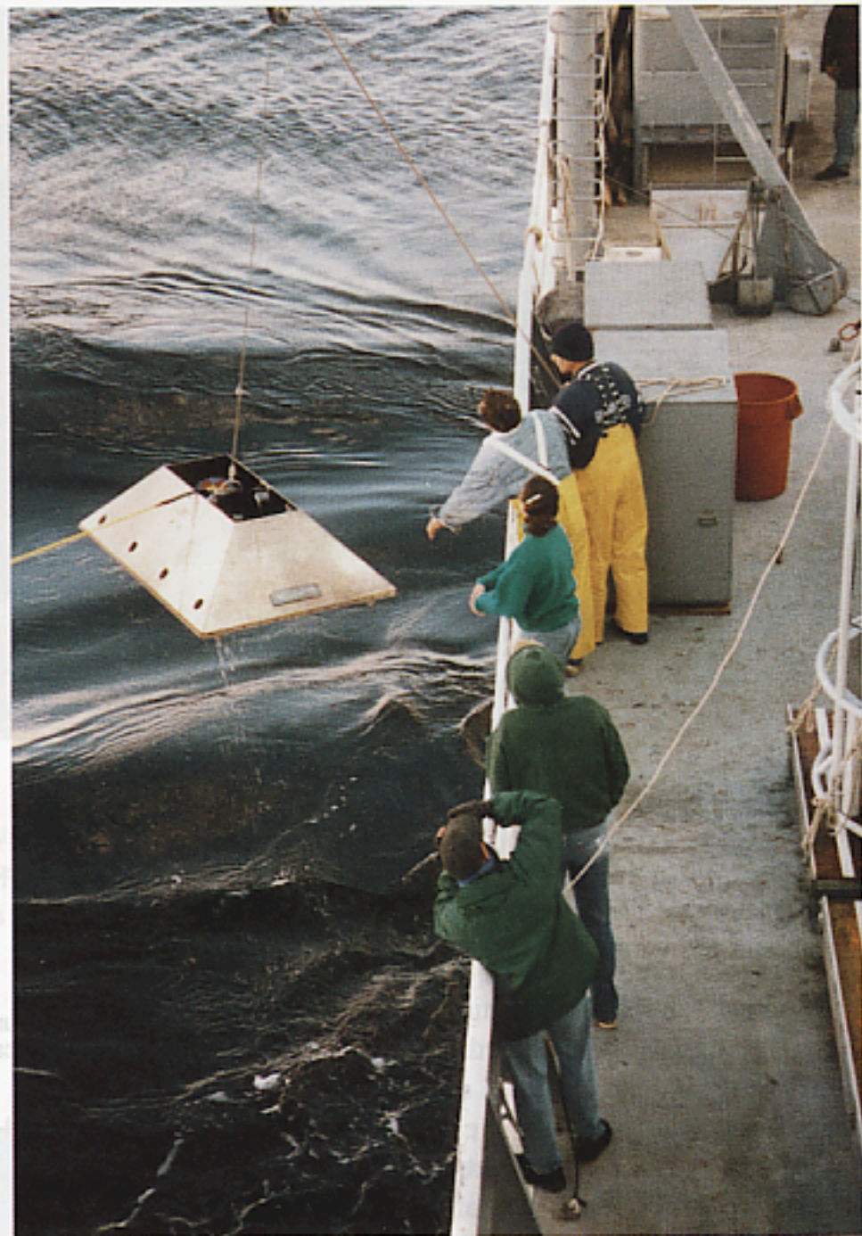
Figure 9.21 Retrieving a Doppler current meter from the sea floor. The sound signals from the meter are analyzed to determine the speed and direction of the current. Courtesy of Mark Holmes, School of Oceanography, University of Washington.
