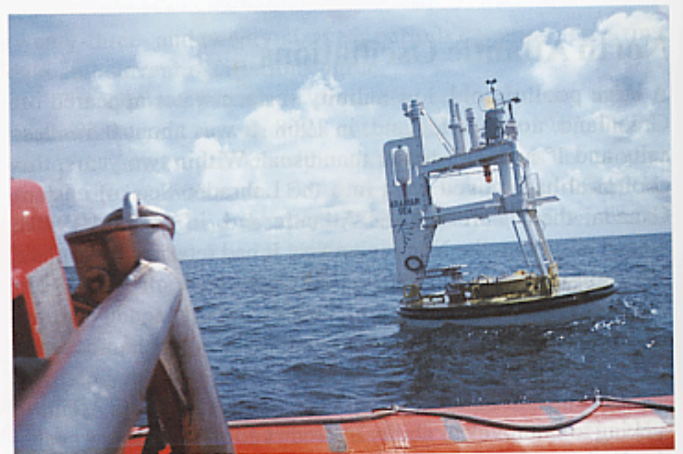
Figure 9.18 Retrieving an oceanographic research buoy in the Arabian Sea (northwest Indian Ocean). This buoy is equipped with weather, radiation, and water property sensors.
