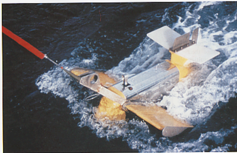
Figure 8.11 Seasoar is a conductivity-temperature-depth sensor that is towed by a ship. The wings allow Seasoar to move vertically while it is towed horizontally.
