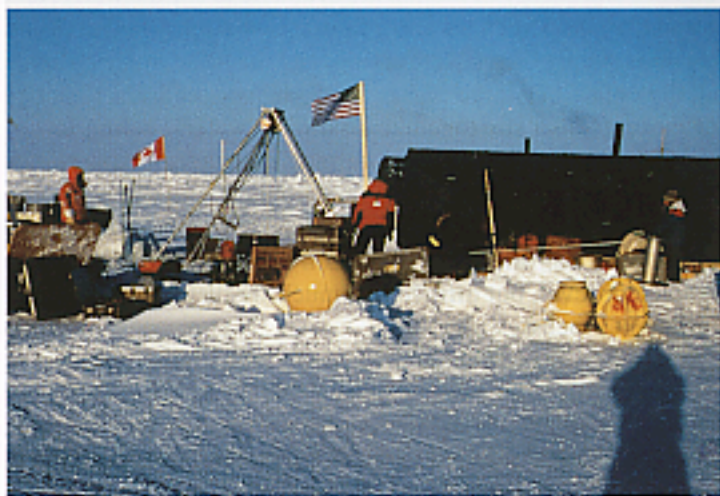
Box Figure 5 The building on the ice combines living quarters and a scientific laboratory. Equipment includes an A-frame and buoys ready for deployment through the ice.
