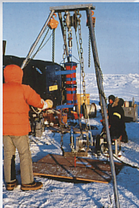
Box Figure 4 Deploying a 4250 m mooring at the North Pole. The mooring is outfitted with a suite of oceanographic instruments. An acoustic Doppler current profiler is located near the top of the mooring.
